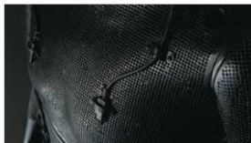
The TOM™ has more than 200,000 sweating holes on its surface, and can measure temperature and humidity within clothing.
